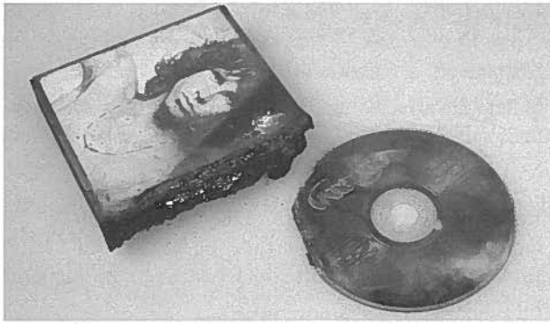
Figure 15. Serious damage can result when CDs are subjected to extreme heat, e.g. from a fire.
